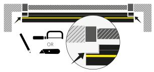
(5) With the door closed, position the floor seal so that the raised section is touching the bottom inside edge of the door.
