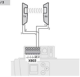
A connected photocell is automatically detected by the controller as soon as the power supply is connected. The photocell can be retrospectively reprogrammed.
