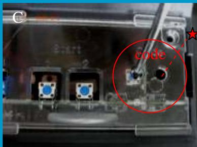
3. Take a small screwdriver press the button as shown in picture C once and release
