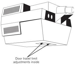
The travel of the door is set by adjusting two screws at the bottom of the opener. These screws are inside the light cover and are marked as up limit and down limit. There are arrows indicating which direction to adjust for more travel in either direction. One full turn of either screw results in around 250mm of trolley travel. Always run the opener to place the door at least 500mm from the appropriate limit before making any adjustment.
