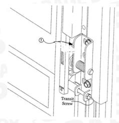
3. Undo the two grub-screws in the cable drum towards the centre of the door. The cable can now be inserted into the fixing slot. Rotate the drum so that the cable winds onto the rear of the drum. Ensure the cable runs down the inside of the track. When the cable is taut, slide the drum to the outside and tighten both grub-screws. Repeat for opposite side if required
