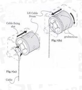
4. Undo the grub-screws that were tightened in step 1
